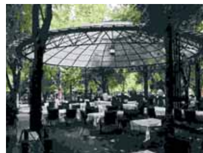
Restaurant Madera in Belgrade chose Lexan Thermoclear sheet for its canopy due to its excellent light transmission, easy installation and UV protection on both sides
